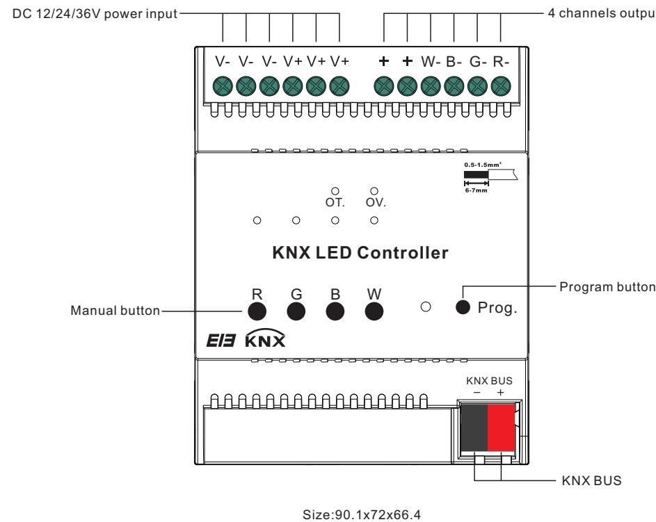
The dimmer with LED constant voltage drive can drive LED directly, has four channels, each channel is independent.
